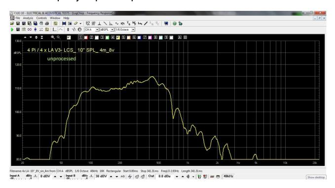
Figure 9a. LO Section - Frequency Response of LO Section of 4xLA V3, free space (4xPi), 8Vrms, at 4m on axis, unprocessed
